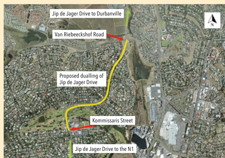
Doubling up: The yellow line indicates the section of Jip de Jager Drive where the City will be adding additional lanes to increase the capacity of this key link between the N1 and the suburbs of Durbanville, Welgemoed and Bellville.
